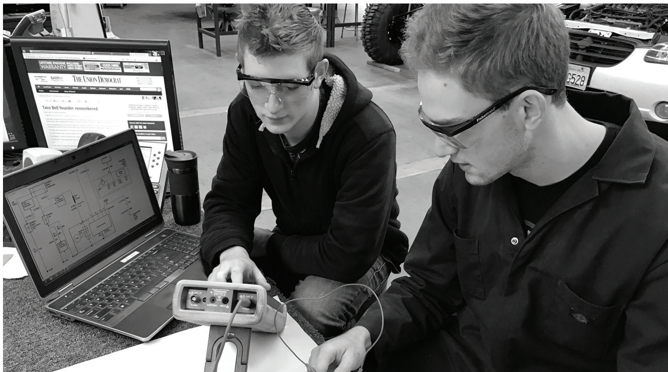
Automotive Technology students check the resistance on an alternator starter using a Fluke meter. Columbia students receive vocational training in the most current industry technologies.
