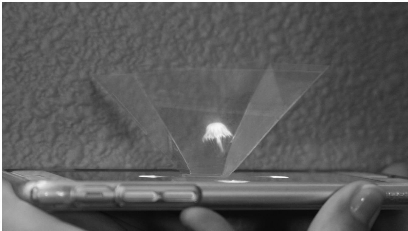
A moving hologram inside a 3D mini Hologram Projector built by Columbia physics students
